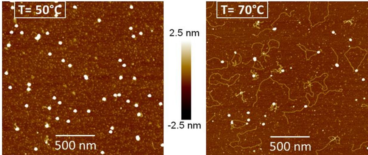
**Figure 2:** Example of AFM image of AAV8 capsids incubated for 15 minutes at 50°C or 70°C. Above 60°C, some single stranded DNA ejected from the virus can be observed. Using image analysis tools, we are able to quantify the length of DNA ejected as a function of temperature and/or time of incubation.
